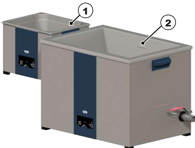
Illustration 5: Elmasonic Select 30–900 fill level marking
